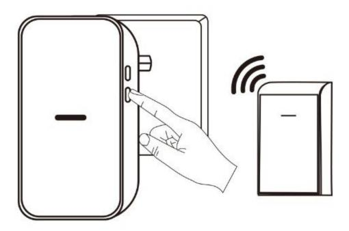
Clear code pairing: If the receiver is disconnected, press and hold the "volume control button", then turn on the power until you hear "bim bam, bim bam", then release your hand to clear all the code pairings in the device, then all the transmitters will disabled and will need to be re-paired.
